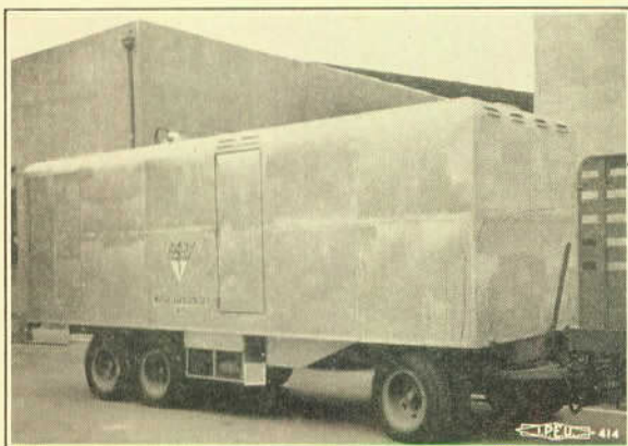
Members of L. U. No. 40 built this rolling motor generator set which has proved itself a mighty handy item in the production of moving pictures.
