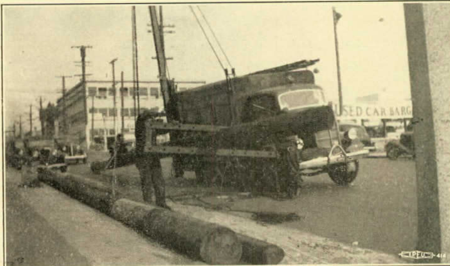
Invention of Brother G. D. Leister of L. U. No. B-1245, a gin pole attached to line truck which greatly facilitates handling poles.
