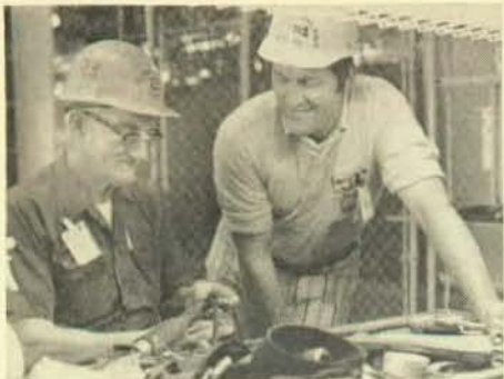
Maintenance electricians at Ingalls keep the facilities and equipment in shape to build ships. Among their jobs is the repair of welding cable, which is being done by Arnold C. Givens, left, a maintenance electrician with five years at Ingalls. Maintenance electrician foreman, Wayne M. Hines, with 13 years at Ingalls, checks the job.
