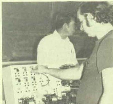
Third year apprentice Bill Parm hooking up a practice motor control board. Instructor Bob Nelson is in the background.
