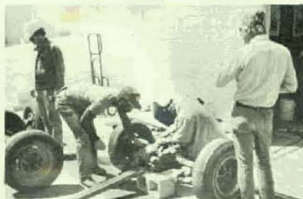
Pictured left to right are Brothers Paul Yates, Jerry Traylor, Harold Carter, and Dale McGarvie starting the PAC 357 trailer project by welding platforms on the axles.
