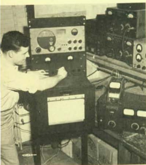
This worker is calibrating radio frequency field-intensity equipment in Bureau of Standards mobile unit.
