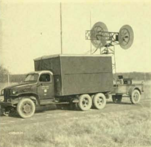
The mobile unit for investigating microwave frequency propagation effects.
