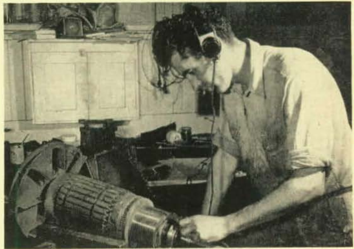
In an L.U. 6 motor shop, Apprentice Adam Brawley learns fine points about motor repair as he tests an armature. The San Francisco apprentice system has had high praise.
